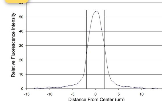
Point-spread function based on the relative fluorescence intensity of an image of a 4-µm calibration microsphere (FocalCheck™, Molecular Probes) corrected for background. The resulting full-width at half maximum (FWHM) is 4.388 µm. Vertical bars indicate the width of the microsphere.
